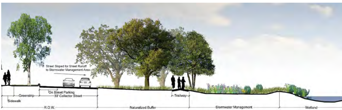
Figure 56. Stormwater Treatment Train within Conservation Development.
